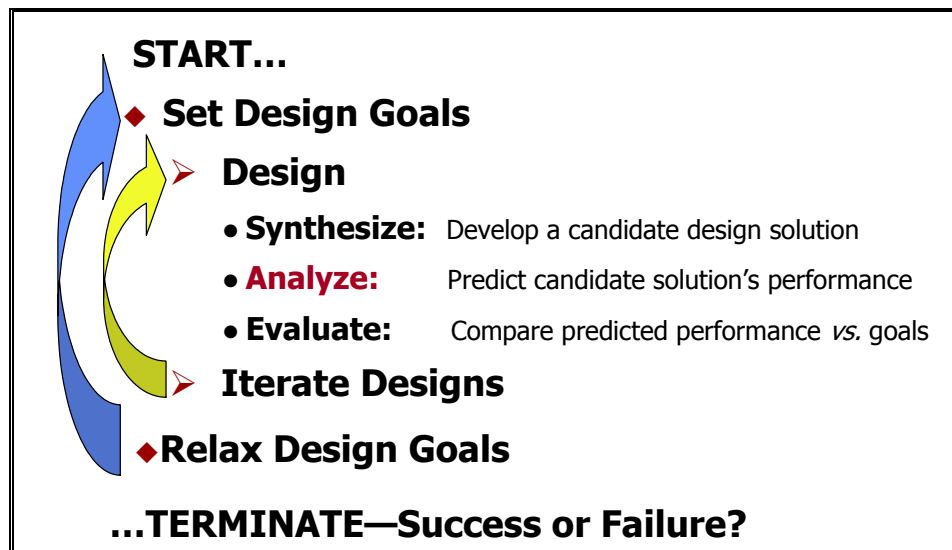
Figure 1. A Formal, Double Loop, Design Process. A designer sets goals for the performance of an artifact, then cycles through the inner design loop, searching iteratively through design alternatives. In each cycle the designer proposes a candidate solution, analyzes it to predict its performance and compares its performance to the current set of goals for the artifact. When an alternative is found that achieves acceptable performance, the process terminates. If no candidate solution can be found whose goals satisfy the required set of goals, the designer enters the outer loop and evaluates whether a reduced set of goals can be found that is still attractive enough to pursue. If so, one or more of the goals are relaxed and the designer reenters the inner loop to search for a solution that meets the reduced set of goals. The design process terminates in success when an acceptable solution is found; or in failure, if no acceptable solution can be found without lowering goals below a threshold of acceptability. Note the close similarity between this view of design and the general model of adaptive search in organizations proposed by Cyert & March (1963; 1992).
